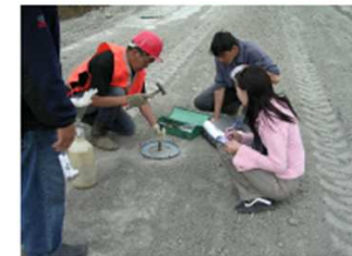
Photo-3.1.27 Field density test
