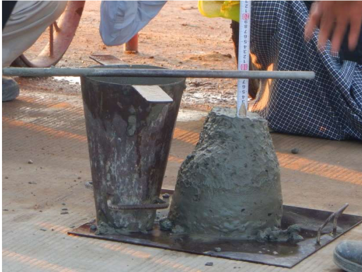
Slump test conducted. Slump 8cm, slightly hard.
